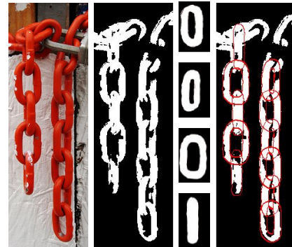
Fig. 1. Separating chain links from the background and from each other by convex optimization in terms of a sparse covering of the image by shape templates. The dictionary of shape templates was generated from four templates by translation, rotation and scaling. The approach presented in this work copes with a significant amount of overlapping templates and occlusion. Left to right : Original image, pre-segmentation using a thresholded distance to the color red as foreground indicator, shape templates used for segmentation, and the final result.
